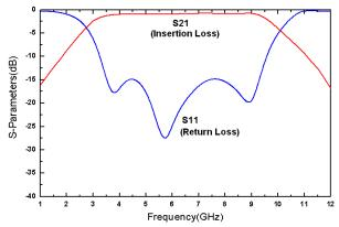
Fig. 4. Simulated results of proposed UWB Filter
