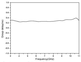
Fig. 8. Measured Group delay
