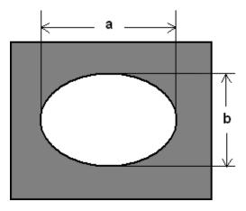
Fig. 1. Elliptic shape slot
