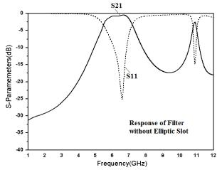
Fig. 5. Simulated results of filter without Elliptic shaped Slot
