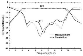
Fig. 7. Measured results of UWB filter
