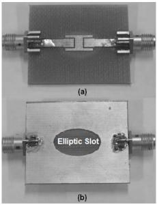
Fig. 6. Photograph of the UWB filter
